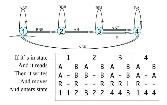
This machine will sort any random string of A's and B's so that all of the A's are listed first, then all the B's. The machine begins by reading the symbol on the far left of the tape.
